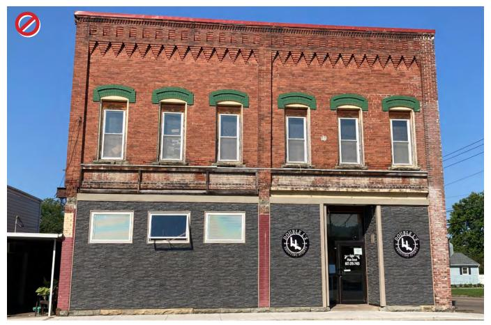
Do not use inappropriate materials such as fake stone veneer to infill storefront windows and reduce transparency into the building.
